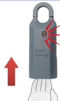
4. When the *Success!* message appears on your eKEY, press up on the bottom of the keybox to release the key container.
