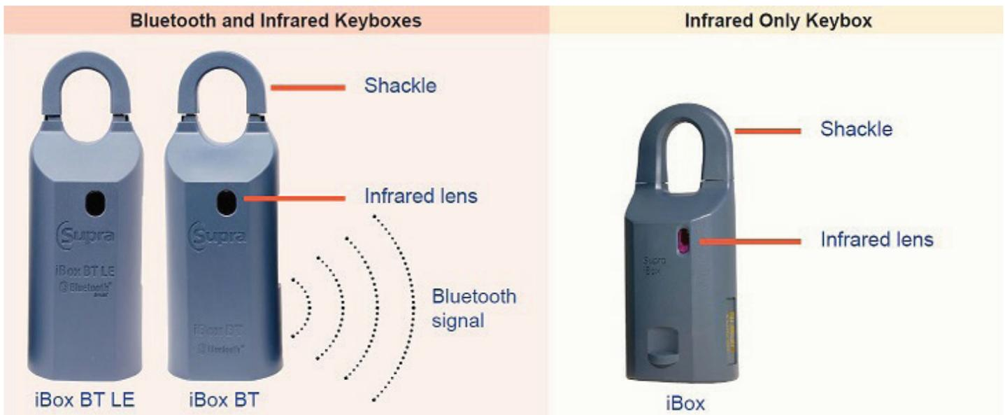
**NOTE: Direct sunlight and Bluetooth signals can interfere with infrared communication signals. It may be necessary to shade the area between the keybox and the fob, or to wait for the keybox's Bluetooth to turn off if it was accidentally turned on (the red LED inside the infrared lens of an iBox BT or iBox BT LE will stop flashing when the Bluetooth turns off).**
